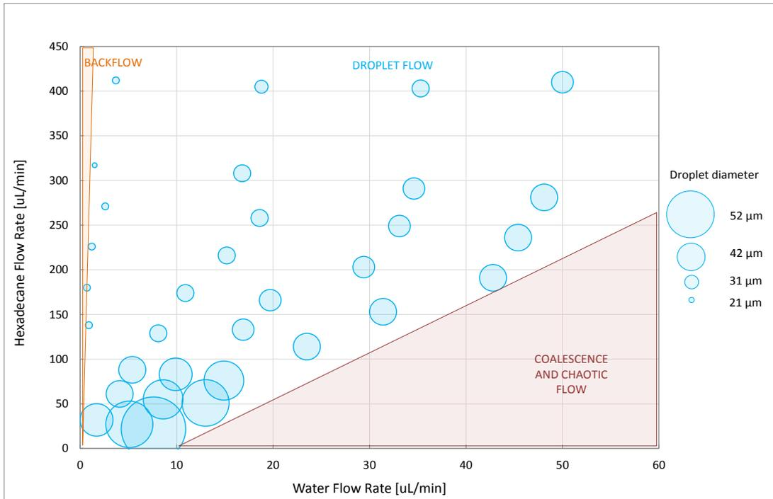
Shown above is information contained in an earlier graphic (relating pressures and droplet size) presented here as a function of fluid flow. This is useful in situations where flow sensors are used in testing setups. Use of in-line flow sensors are always recommended in order to better characterize and thereby optimize test conditions.
