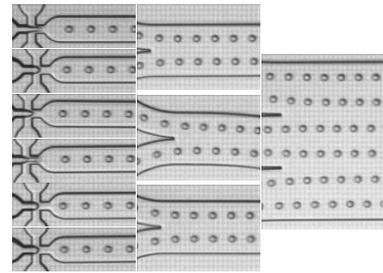
The system is based around a standard Dolomite chip with a series of parallel droplet junctions producing water-in-hexadecane droplets. Flows rates of both fluids are controlled via Dolomite P-Pumps providing pulseless flow. The resulting droplet size and frequency is varied to explore the operating boundary of the system.
