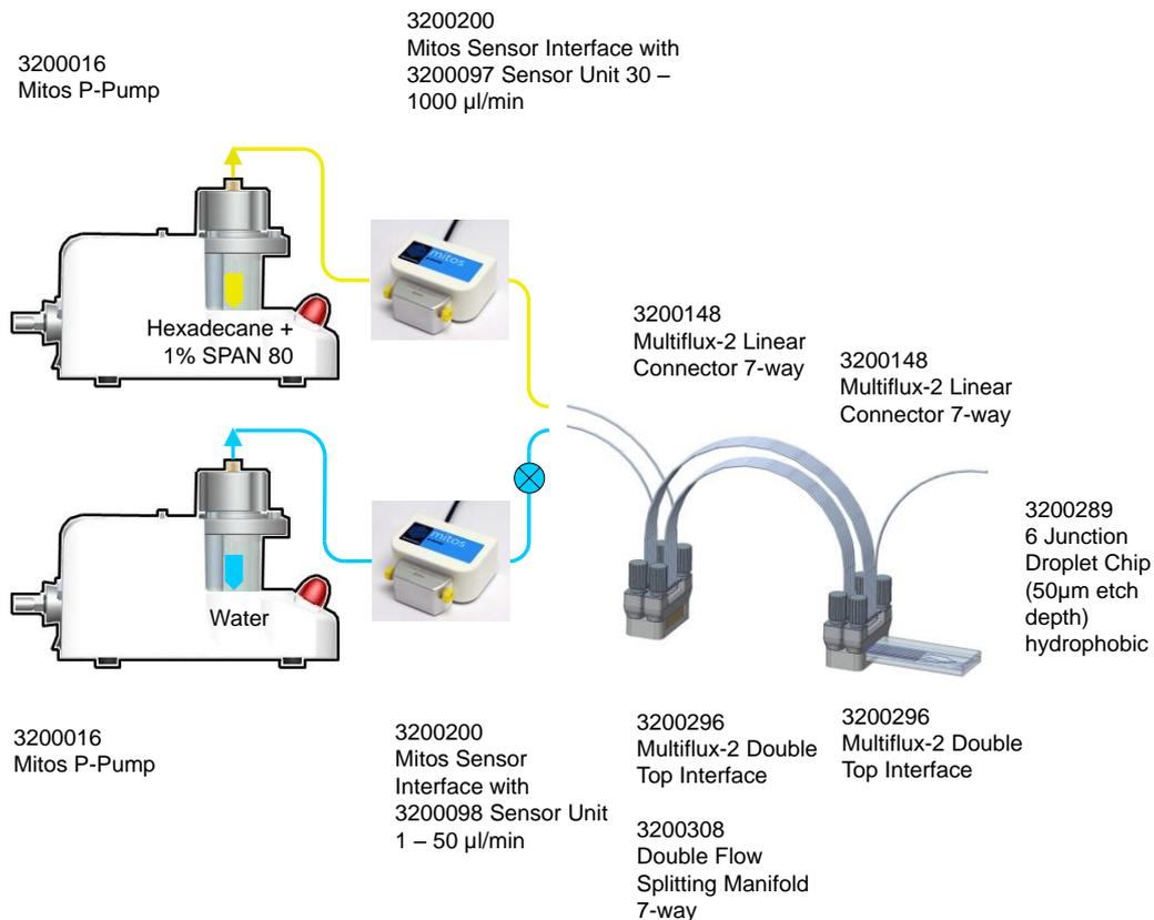
Flow resistors enable the system to be used in an exploratory mode. By suitably selecting flow resistors, a droplet system may accommodate fluids with a wide range of viscosity. Suitable lengths of tubing are cut as flow resistors and connected in the setup as shown in the block diagram below. The resistances are selected based on calculations performed using fluid properties of Hexadecane (with 1% SPAN 80) and Water.
