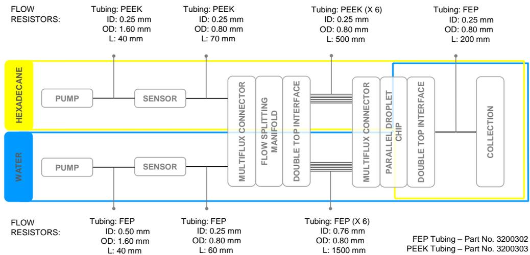
With a change of fluids, the tubing is easily modified to change the flow resistance, thereby enabling quick parametric variation. Additionally, the ability to tune resistances in the system allows for higher resolution in fluid control. 12 resistors interface between the connectors to enable desired flow rates. A brief description of leveraging resistors to tune droplet setups is presented in Appendix C.
